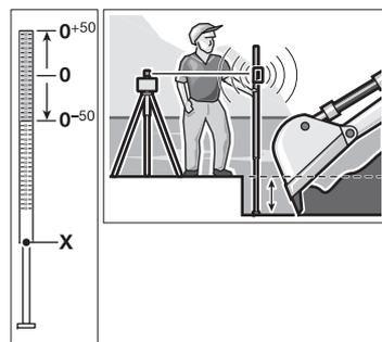
A relative millimetre scale ( $\pm 50$  cm) is marked on the top of the measuring rod **31**. Its zero height can be preset at the bottom of the elevator column. This allows for direct reading of deviations from the specified height.
