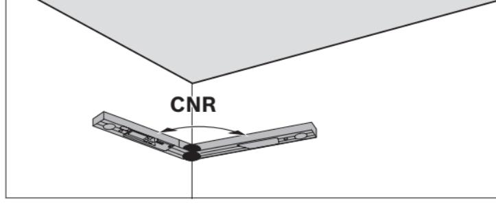
To measure the corner angle, place the fold-out and base legs flat against the walls and read the measured corner angle or set a known corner angle on the anglefinder.
