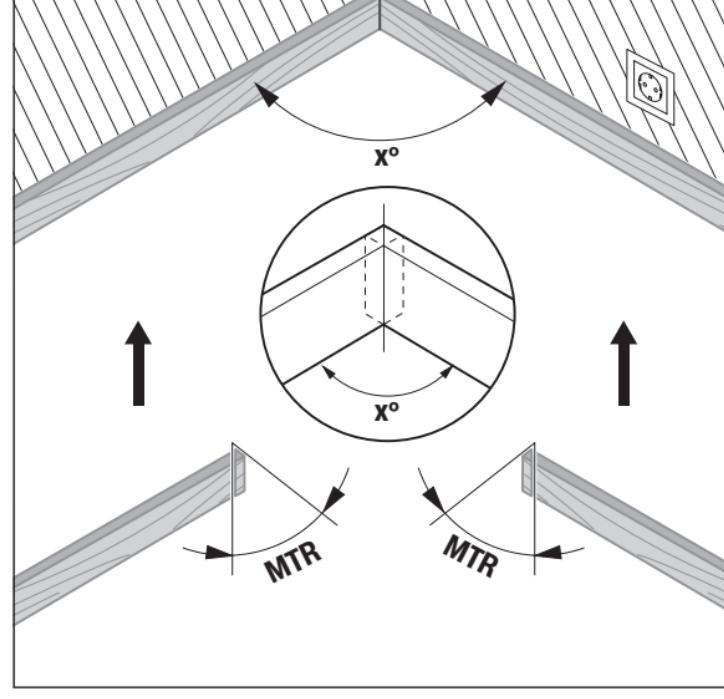
The miter angle “**MTR**”, by which the two workpieces are to be shortened, is calculated. For these miter cuts, the saw blade is vertical to the workpiece (the bevel angle is 0°).
