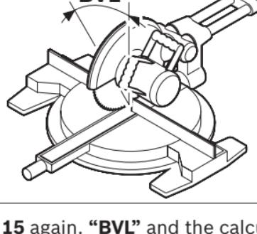
Press button **15** again. “**BVL**” and the calculated bevel angle for the chop and miter saw is indicated on the display.
