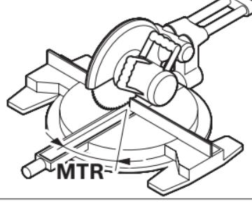
Press button **15** again. “**MTR**” and the calculated miter angle for the chop and miter saw are indicated on the display.
