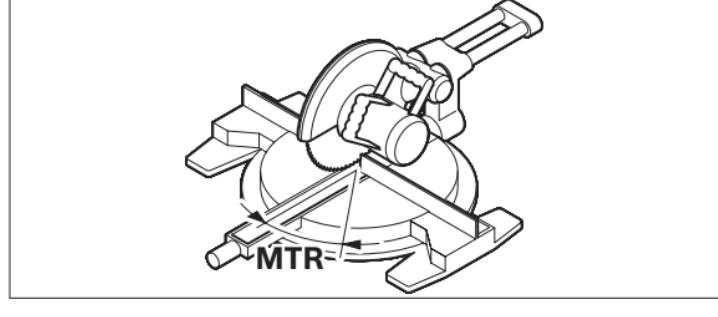
Press button **14**. The calculated horizontal miter angle “**MTR**”, which has to be set on the chop and miter saw, and the “**MTR**” indicator will be shown on the display.
