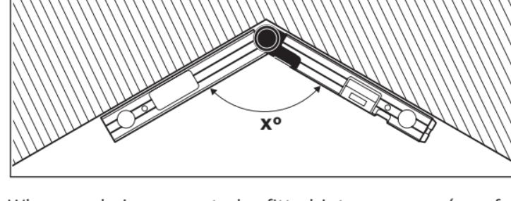
When workpieces are to be fitted into a corner (e.g. for floor trimmings), measure the corner angle **x°** by applying the fold-out leg and the base leg. For given angles (e.g. picture frames), open the fold-out leg and the base leg until the desired angle is indicated in the display.
