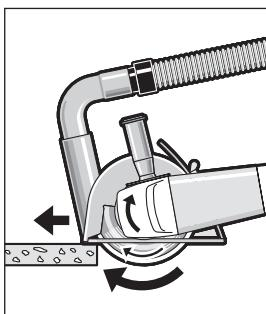
Switch on the machine and place the front part of the cutting guide on the workpiece. Slide the machine with moderate feed, adapted to the material to be worked.
