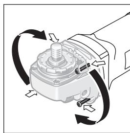
The machine head can be rotated with respect to the machine housing in 90° steps. In this manner, the On/Off switch can be brought into a more convenient position for special working situations, e.g. for left-handed persons.
